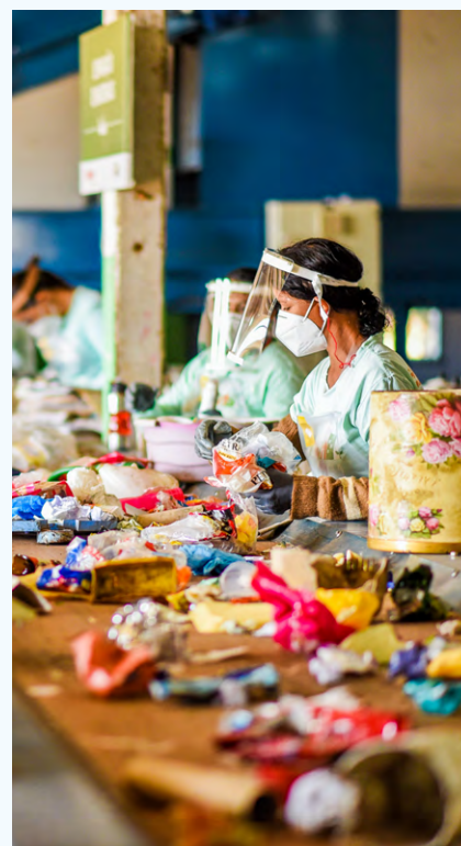
Recyclable materials are manually separated into recycling streams on the sorting line.
